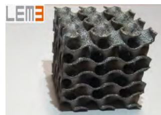
Fig. 3. Fabricated TPMS-based lattice.
