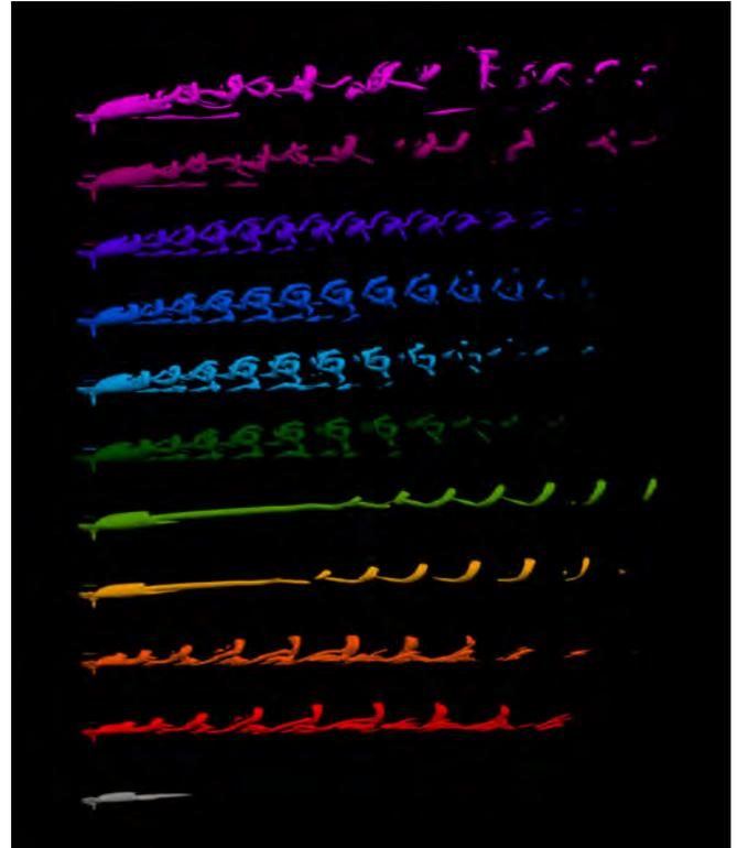
**Figure 2:** Isocontours of vortex visualization quantity for different jet inflow velocity ratios. From top to bottom:  $R = [0.9, 0.8, 0.775, 0.75, 0.7, 0.6, 0.5, 0.4, 0.375, 0.35]$
