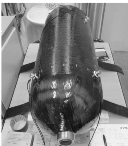
Fig. 1. Hydrogen pressure vessel prepared for acoustic emission testing.
