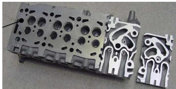
Fig.1. A diesel cylinder head of PSA Peugeot Citroën
