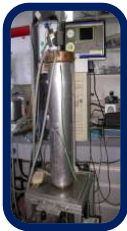
Fig. 1. High Temperature - High Pressure (HTHP) polymerization device.
